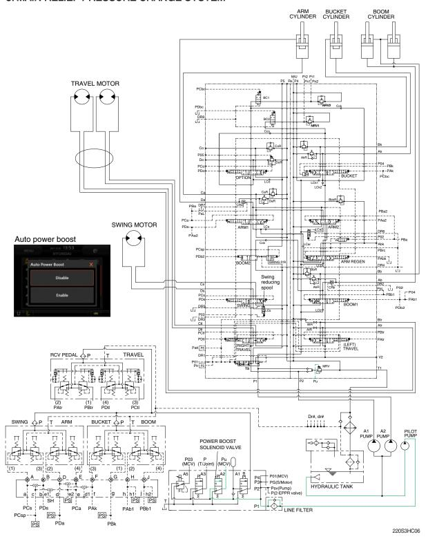
When the power boost switch on the left control lever is pushed ON, the power boost solenoid valve is actuated, the discharged oil from the pilot pump flows into **Pu** port of the main relief valve of main control valve; then the setting pressure of the main relief valve is raised from 350 kgf/cm² (4980 psi) to 380 kgf/cm² (5400 psi) for increasing the digging power.
